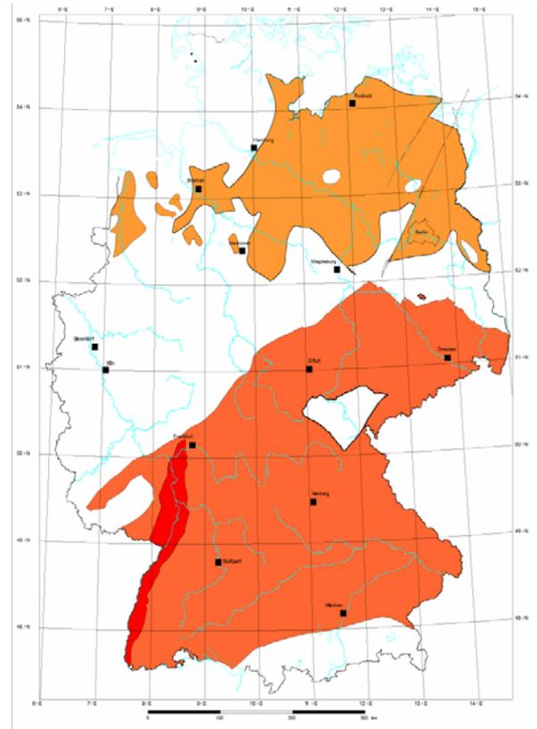
**Figure 3:** Crystalline rocks for geothermal power production in Germany. Red area: crystalline rock at 3 km depth and with a mean temperature of 100 °C; dark red area: crystalline rock in the Upper Rhine Graben at 3 km depth and with a temperature of 130 °C; orange area: Rotliegend (Permian) volcanic rock with temperatures exceeding 100 °C.
