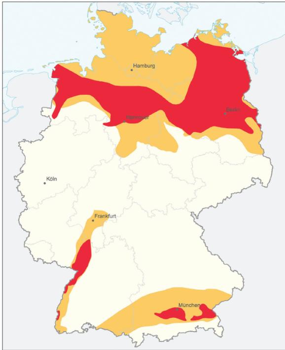
**Figure 1:** Red areas: Hot water aquifers for geothermal power production, temperature above 100 °C. Yellow areas: Hot water aquifers direct use of geothermal energy, temperature above 60 °C. (Schulz et al. 2007). From North to South: Upper Rotliegend (Upper Permian) sand stone aquifer in the North German Basin; Upper Muschelkalk and Buntsandstein (Middle and Early Triassic) aquifers of the Upper Rhine Graben; Malmkarst (Upper Jurassic) aquifer in the South German Molasse Basin.
